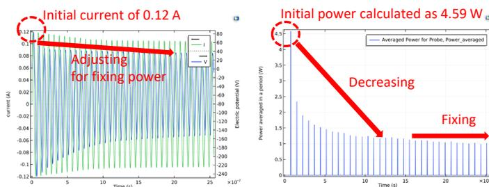
Figure 1. Time-dependent current/voltage profiles (Left) and power averaged at the end of each period (Right) for the first few periods.
