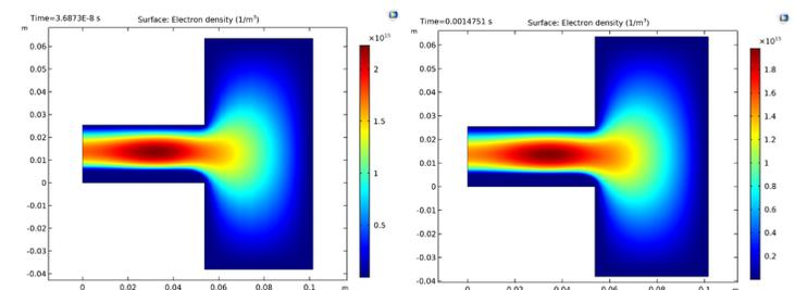
Figure 4. Electron density distributions obtained using Time Periodic to Time Dependent study (Left) and Time Dependent study (Right), respectively.
