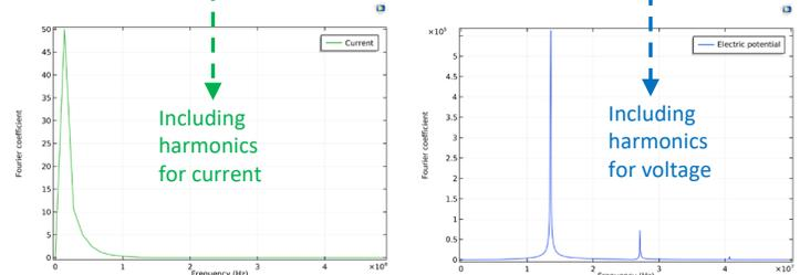
Figure 3. Fourier transform of the current in the time-periodic (Left) model and that of voltage in the time-dependent (Right) model, respectively.
