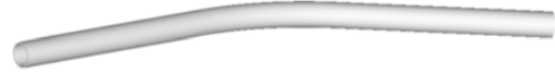
Figure 8: Curved pipe (25°, radius of curvature 26 m): pipe diameter equal to 2 m, mean velocity equal to 3.63 m/s.
