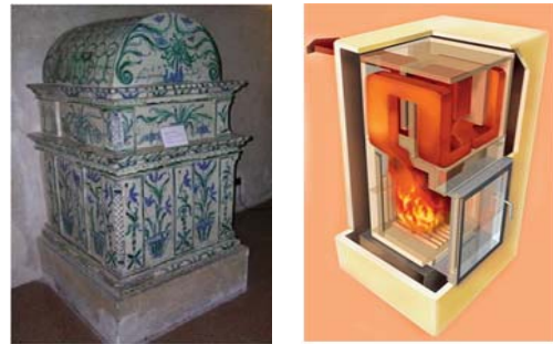
Figure 1: Left: historical "Sfruz" heat accumulation stove, located in the Buonconsiglio Castle in Trento, Italy. Right: view of a project design of modern stoves, where can see combustion chamber and twisted conduct.
