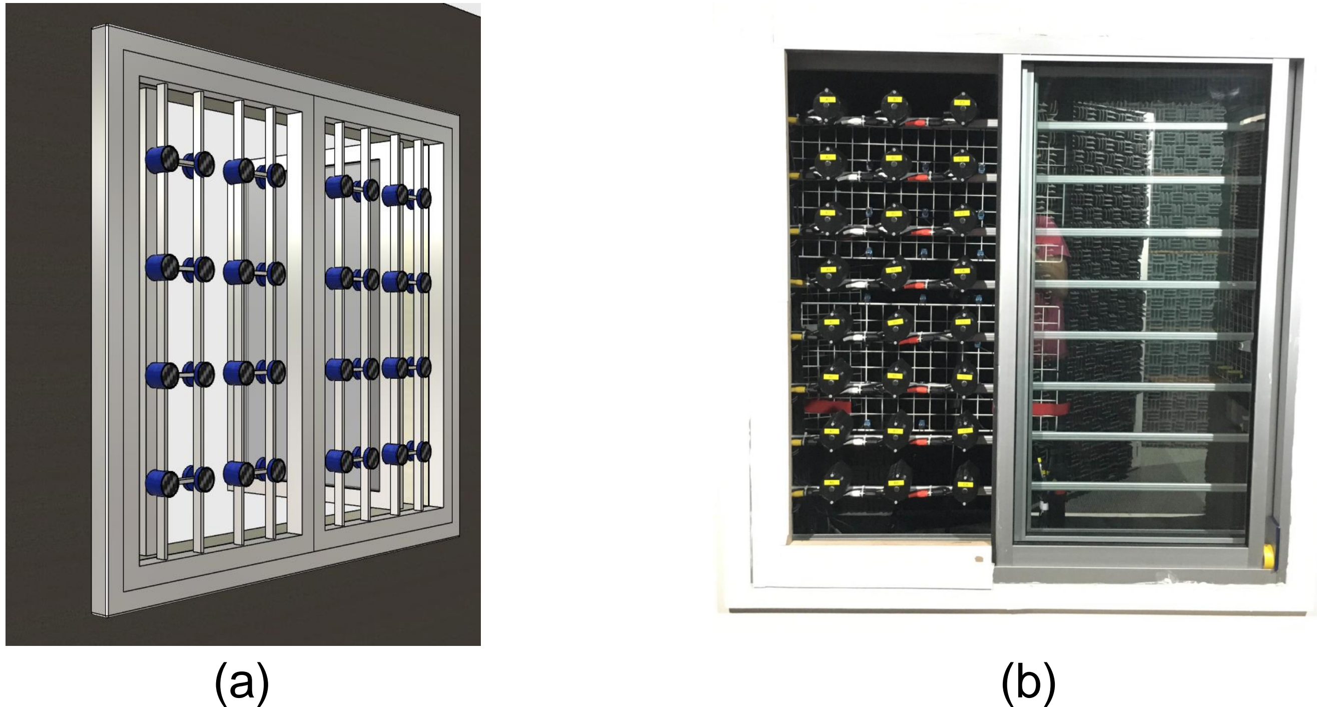
Figure 1. (a) Proposed acoustic window based on the active noise control concept. (b) Acoustic window prototype designed in Nanyang Technological University.
