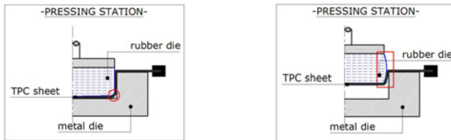
Figure 2 Rubber deformation (left side), barreling effect of rubber (right side).
