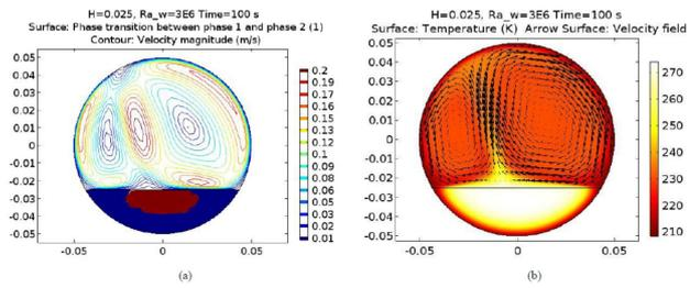
**Figure 1:** (a) Phase contours (blue: solid, red: liquid) and air circulation above it, and (b) velocity arrow and temperature contours at  $Ra = 3 \times 10^6$ , filled percentage = 25% and time = 100 s.
