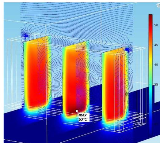
**Figure 7.** Cross sections areas of temperatures (°C) and electric field shape (blue contours) at  $t=80s$  (local maximum of temperature is located at the bottom side of the water sample)
