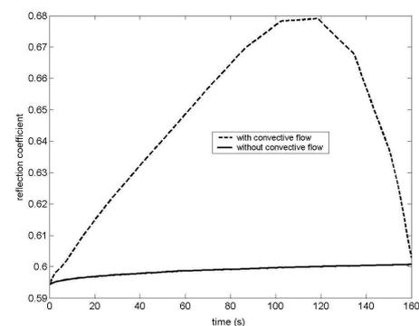
**Figure 9.** Reflection coefficient as a function of processing time.
