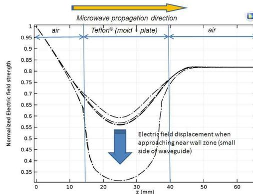
**Figure 4.** Electric field distribution (normalized) within the waveguide filled with the PTFE support as a function of microwave propagation direction.
