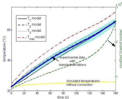
**Figure 8.** Simulated temperatures from  $T_1$  to  $T_3$  (black) and max temperature (red) vs. experimental measurements (blue) with standard deviations (cyan) as a function of processing time (left y-axis), modified Grashof number (right y-axis)
