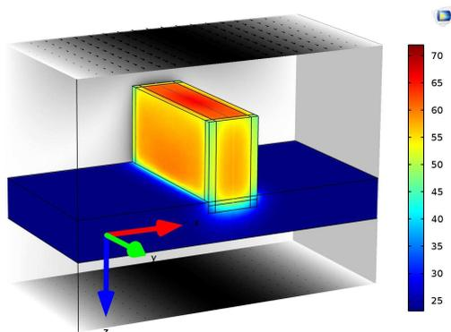
**Figure 5.** Temperature distribution (°C) within water and PTFE support plate at  $t=160s$
