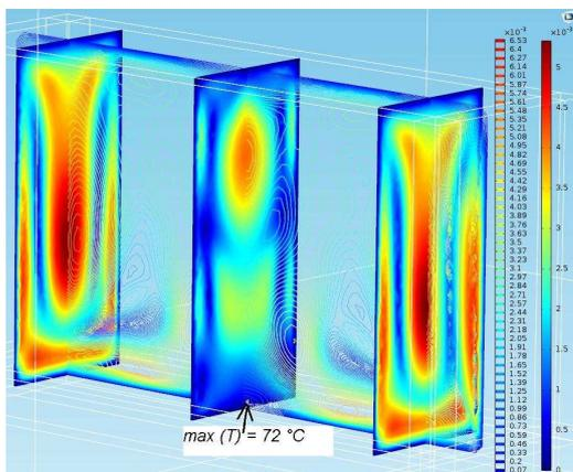
**Figure 6.** Cross sections areas of velocity fields (m/s) at  $t=160s$  (local maximum of temperature is located at the bottom side of the water sample)
