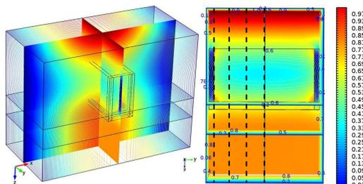
**Figure 3.** Electric field distribution (normalized) within the waveguide filled with the PTFE support: 3D distribution map (left), 2D cross section in  $y, z$  plan (right)
