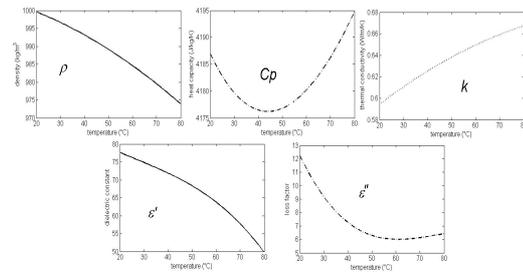
**Figure 2.** Thermophysical properties ( $\rho$ ,  $C_p$ ,  $k$ ) and dielectric properties ( $\epsilon'$ ,  $\epsilon''$ ) for pure water within the range [20; 80 °C].
