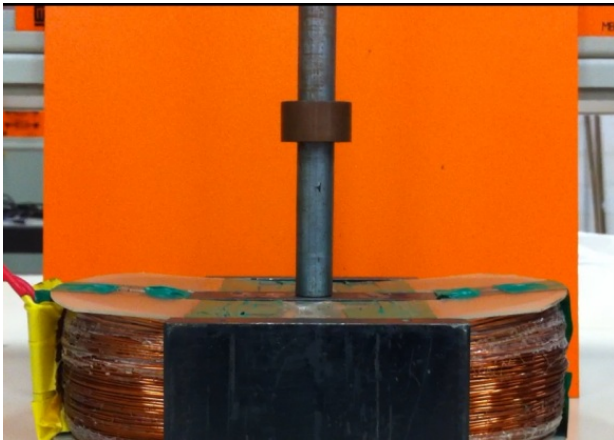
Figure 3: Levitation of copper ring at 127 V and 15 Hz.
