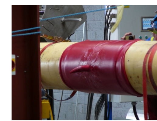
Field joint Needs cooling
