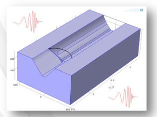
Making reference to the foundation domain, a global ordinary differential equations problem has been solved to compute the displacements associated to the earthquake motions
