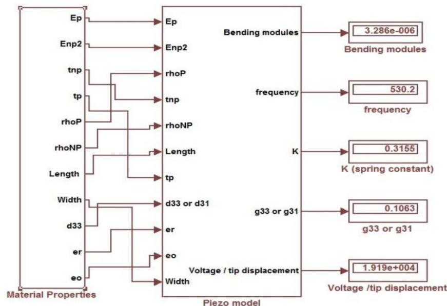
Fig. 1 Simulink model of piezoelectric unimorph cantilever
