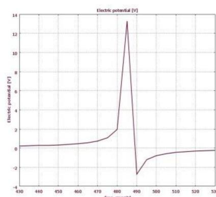
Fig. 3 Frequency Response of piezoelectric micro cantilever
