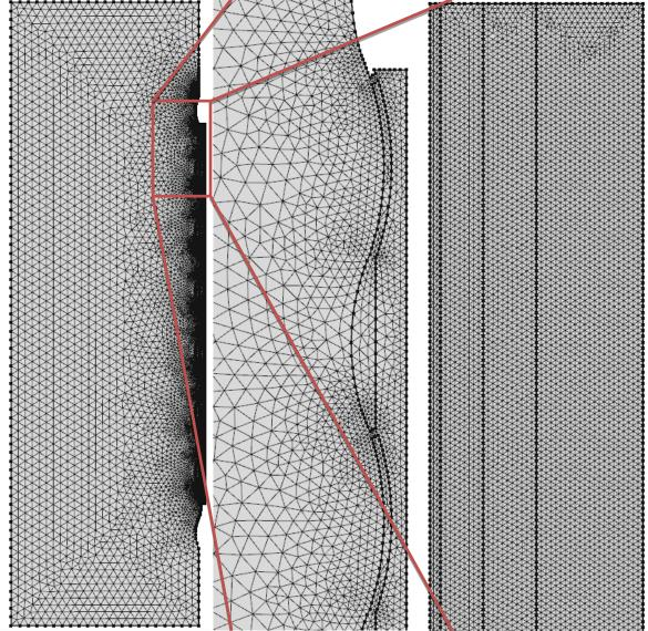
**Figure 14:** Mesh of design 4A with curved facade elements.
