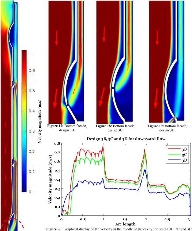
**Figure 20:** Graphical display of the velocity in the middle of the cavity for design 3B, 3C and 3D for downward flow.
