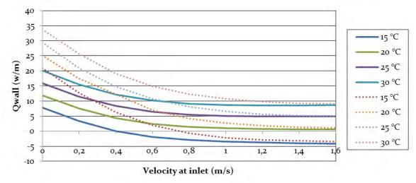
Figure 4: Graph of the heat transfer at the inside of the internal wall to the room, set off to the velocity at the inlet (dotted lines are  $800 \text{ W/m}^2$ ).
