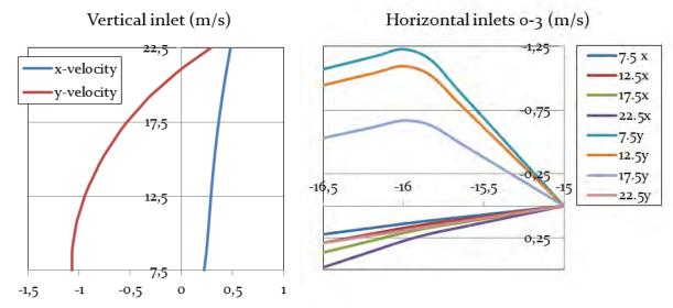
**Figure 9:** Velocity (m/s) measured at 1.5m from the façade at a height of 7.5m-22.5m
