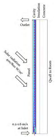
Figure 3: Schematization of the heat balance model
