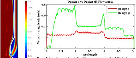
Figure 7: Velocity along the middle of the cavity for design 0 and 3H for downward flow.
