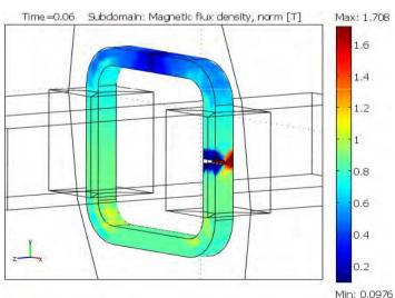
Snap-shot at i<sub>1</sub>(t) = 0 with still high induction level close to the partial gap (right) resulting from the phase shift of secondary current
