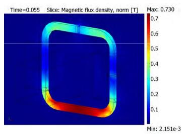
Influence of demagnetizing fields from the full air gap (top) and the secondary windings at i<sub>1</sub>(t) = i<sub>1,max</sub>
