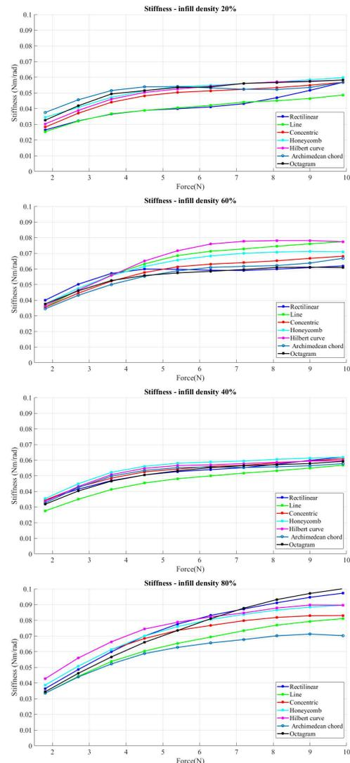
**Figure 6.** Stiffness variation due to different pattern types while keeping the same infill density
