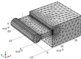
**Figure 3:** FEM discretization of the modular element.
