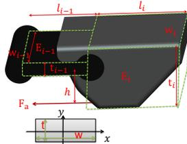
**Figure 2:** modular element of the gripper, composed of a rigid link and a passive elastic element. Main geometrical parameters.
