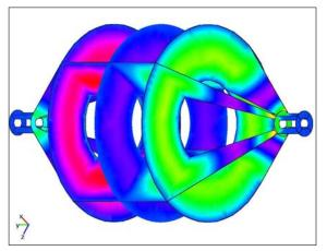
At second TM<sub>01</sub> resonance  $f_{\text{TM}_{012}} = 4.9 \text{GHz}$
