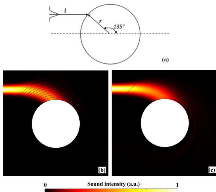
**Figure 1:** (a) Schematic diagram of the incident angle. (b), (c): respective intensity fields of the accurately designed and simplified TGAOA schemes with an incident 13000 Hz Gaussian wave.
