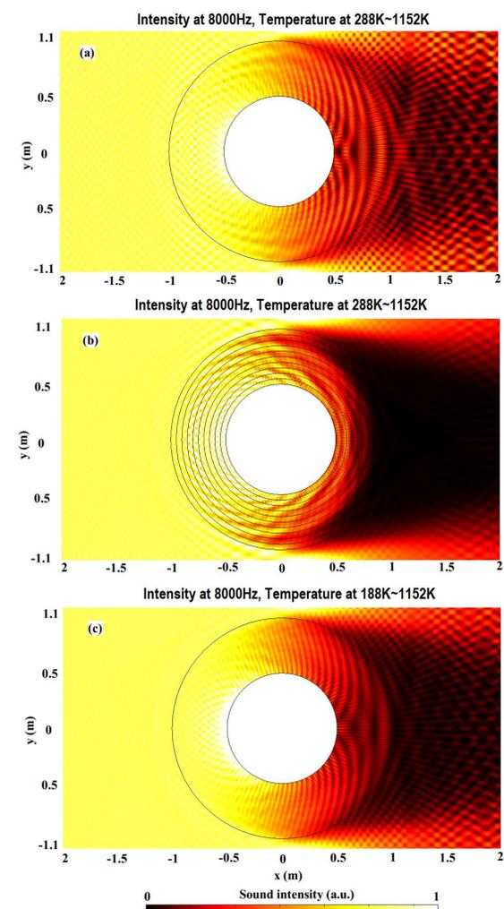
**Figure 2 :** (a), (b): respective intensity fields of simplified and accurately designed TGAOA schemes with an incident 8000Hz plane wave. The temperature at the inner radius is 288K; the one at the outer radius is 1152K. (c) Intensity field of simplified TGAOA schemes with an incident 8000Hz plane wave. The temperature at the inner radius is 188K; the one at the outer radius is 1152K.
