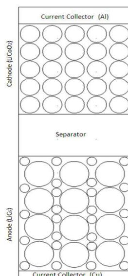
Figure 1: 2-D-Model of Li-Ion Cell.
