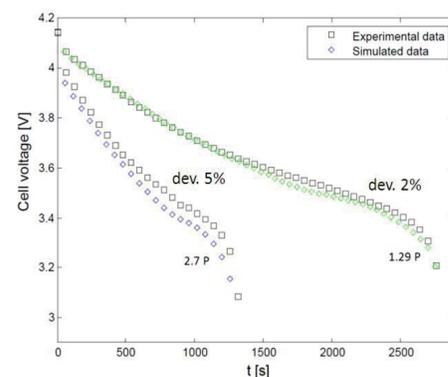
Figure 2: Comparison of simulated and experimental voltage discharge profiles. Deviations of 2-5 % between both validate the model's applicability for different P-Rates.
