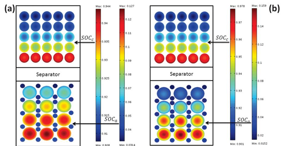
Figure 4: SOC distribution at anode and cathode at 3.2 V for (a) 1 P-Rate, (b) 2 P-Rate.
