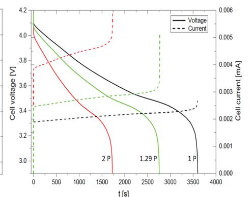
Figure 3: Simulated behaviour of the current and voltage profiles during discharging at different P-Rates.
