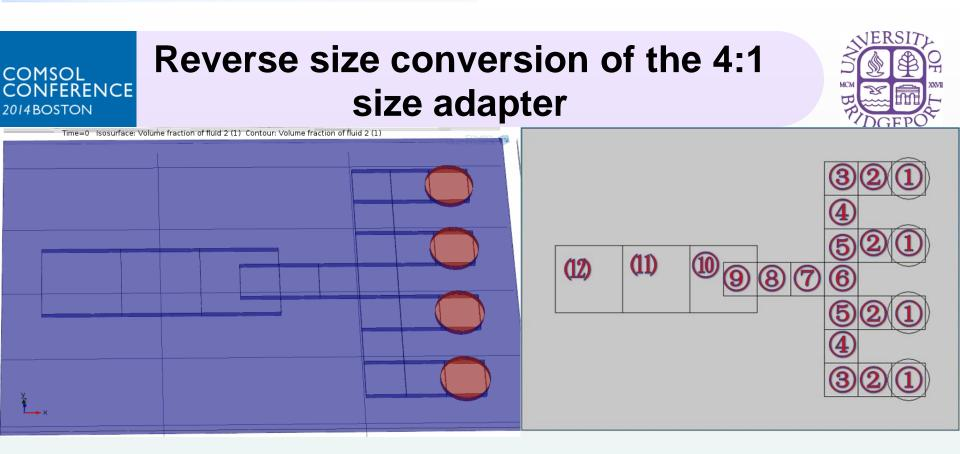
The proposed microfluidic size adapter is bi-directional. When the voltage pulses are applied in the reverse sequence, it can also convert the droplet size in the opposite direction.
