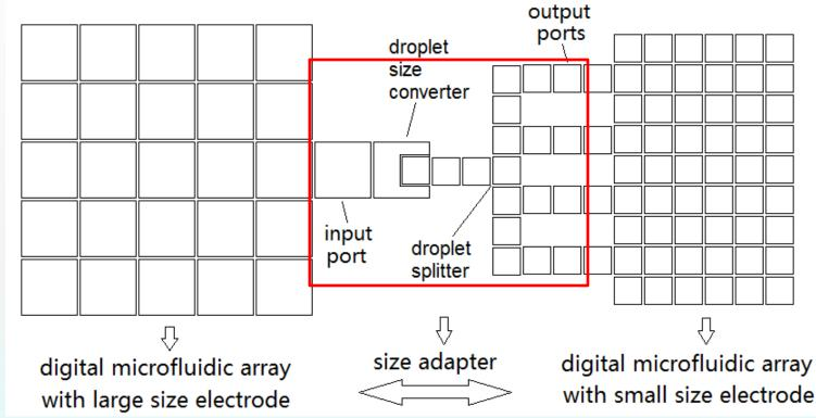
The proposed digital microfluidic droplet size adapter for interconnecting DMFB chips is shown in Figure. It includes input port, droplet size converter, T-shape droplet splitter, and several output ports. The droplet size converter consists of a large electrode with a small electrode embedded inside of it.
