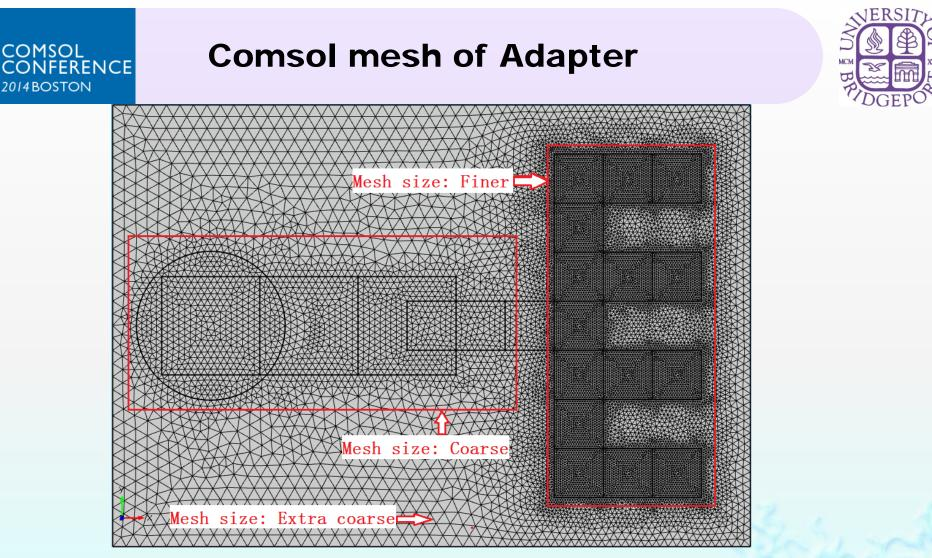
To study this adapter and retain the result more accurate. The mesh model of adapter is shown in the figure.
