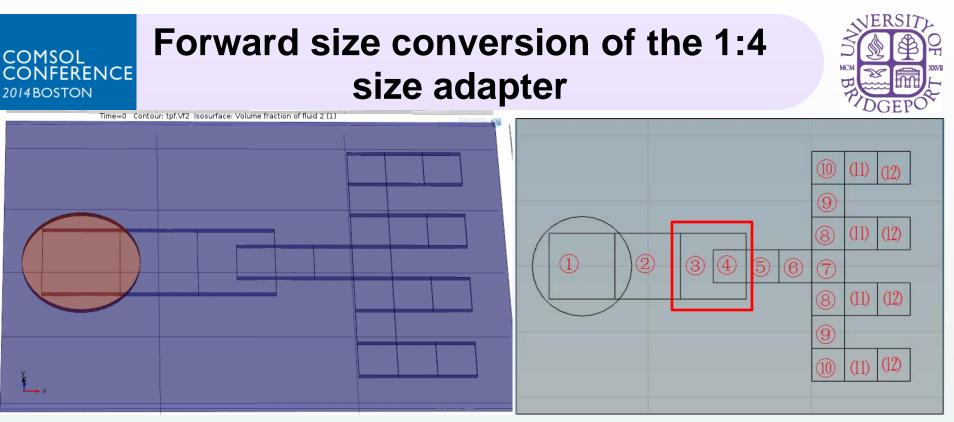
The order of the applied voltage pulses are clearly listed in each electrodes as circled numbers. It requires totally 12 consecutive stages of voltage pulses to complete the size conversion process.
