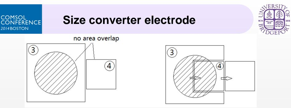
The key part of this size adapter is the size converter electrode: a large size electrode (marked with number "3" in Figure 8) with embedded small size electrode (marked with number "4") along its right side.
