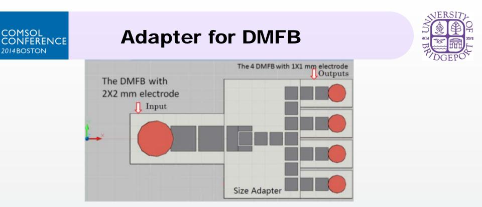
Based on the understanding in COMSOL simulation of droplet moving/merging/splitting, we designed and simulated the microfluidic droplet size adapter, as shown in Figure.
