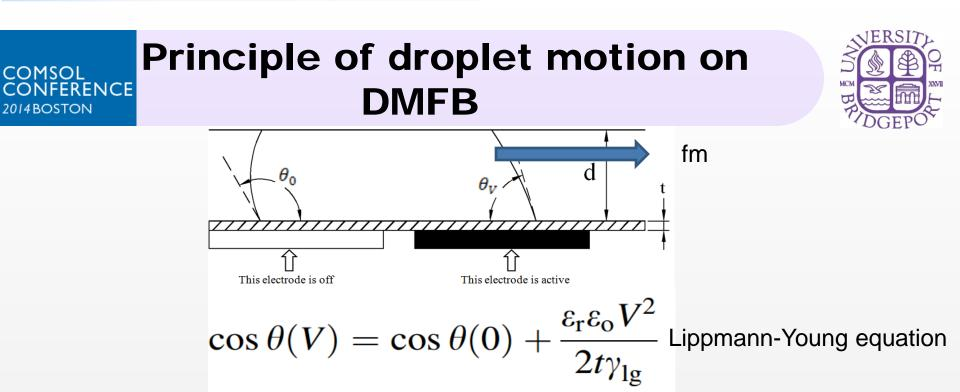
Where  $\varepsilon_0$  (8.85 E-12 F/m) is the permittivity of vacuum,  $\varepsilon_r$  is the dielectric constant of the insulator layer, V is the applied voltage,  $\theta(0)$  is the non-actuated contact angle, and  $\theta(V)$  is the droplet contact angle when voltage V is applied,  $\gamma$ Ig is the liquid-gas interfacial tension.
