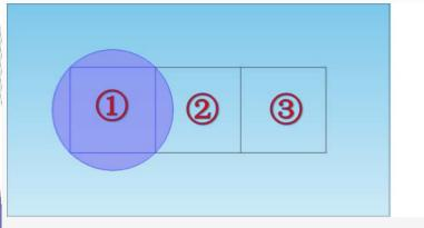
To achieve the movement of droplet on DMFB, at least need three independent control wire to control the condition of electrode.
