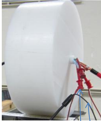
Photo of PE phantom with electrical wiring for thermistors
