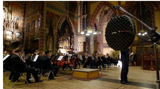
Figure 2. A Jecklin disk employed for a classical music recording.
