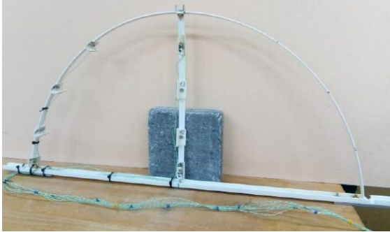
Figure 7. The cross support of thermocouples.
